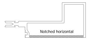
B.) Notch bottom of horizontal for drop-in assembly where required. Reference S-5600 standard installation instructions.
