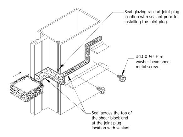
Note: The joinery of the sealant at this area is CRITICAL.
